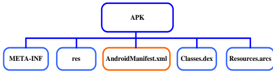
Figure 3. An Android Application Package
