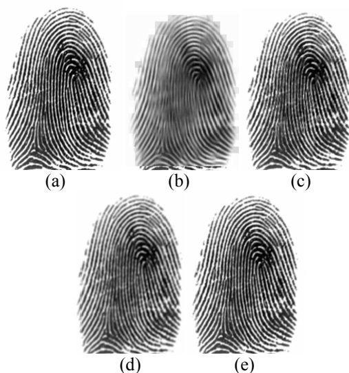
Figure 4.5. Resulted image of (a) original image; filtered with (b) Gabor filter; (c) Median filter; (d) Mean filter; and (e) Gaussian filter.
