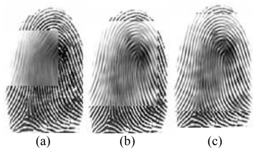
Figure 4.4. Enhanced image resulted by input image of size (a) 150*150; (b) 250*250; (c) 300*300; with mask size of 32.
