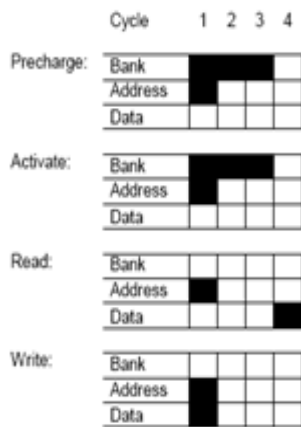
Figure 3. Simplified state diagram and resource utilization governing access to an internal DRAM bank.
