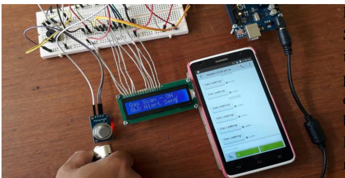
Fig. 13 The implemented system of the warning state that sends “Gas Leaking” message to the pre-defined mobile number.
