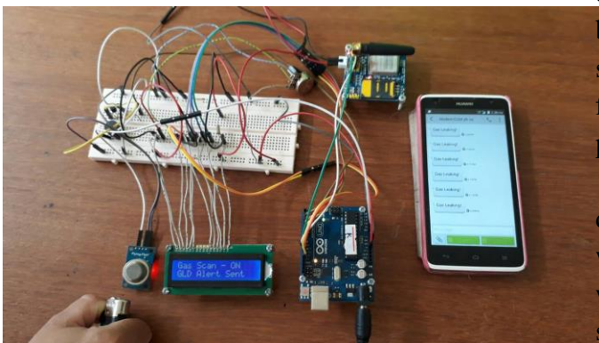
Fig. 12 The implemented circuit of the gas leakage detector using arduino and GSM module with SMS alert and sound alarm when it is in warning state.
